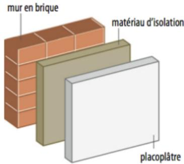
$$R_{th}^{\text{total}} = R_{th}^{\text{mur}} + R_{th}^{\text{isolant}} + R_{th}^{\text{placo}}$$
